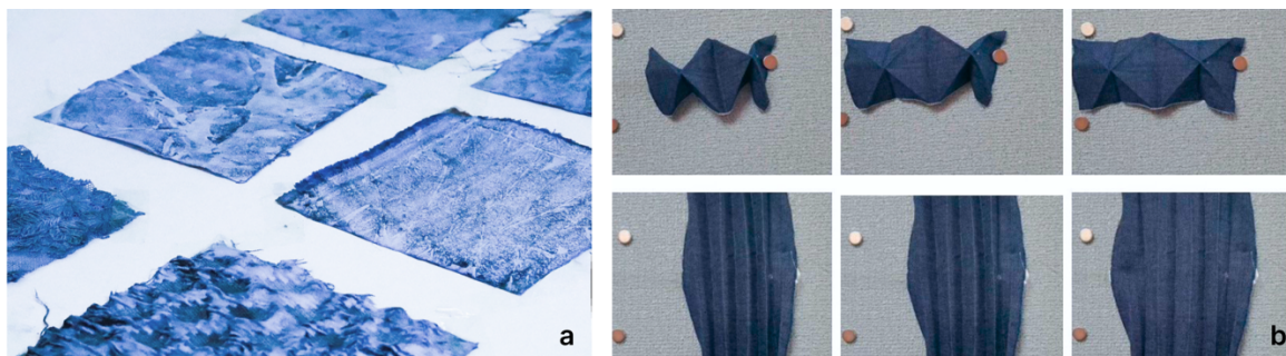
Figure 2: (a) Electromagnetic responsive textile (combined with blue dye). (b) Electromagnetic responsive textile maintains the characteristics of the original fabric and has magnet absorption.
